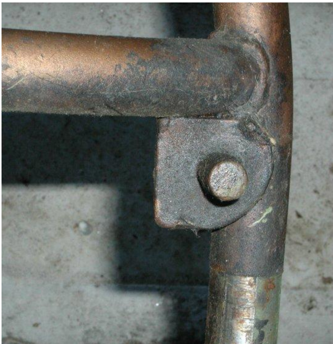
A picture of the stock side stand lug on a 1971 frame, looking at the bottom of the bracket.
