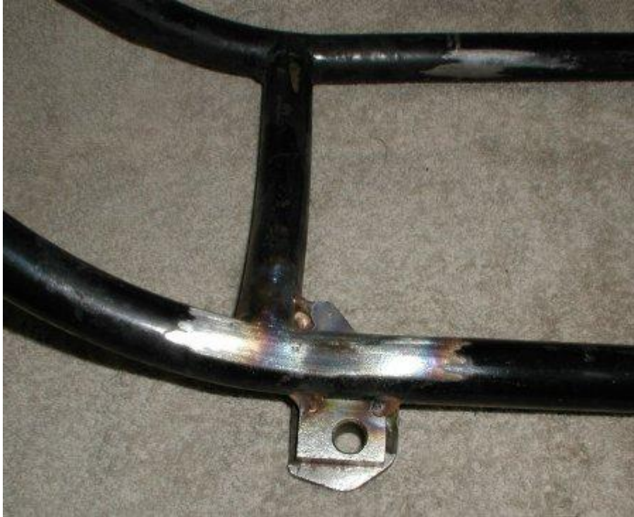
A picture of a frame with the new bracket installed.
