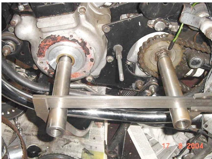
Using a pair of ground centres to check shaft alignment. This accurate method of measurement reveals that the majority of shafts run far from parallel.
