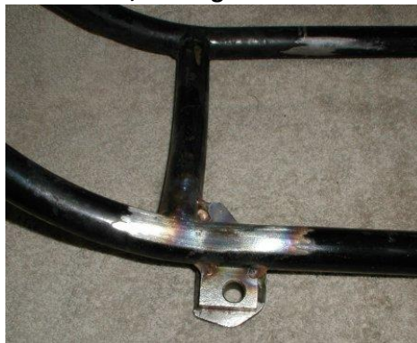
Photo 1: The stock side stand lug on a 1971 frame, looking at the bottom of the bracket.
