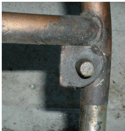
Photo 1: The stock side stand lug on a 1971 frame, looking at the bottom of the bracket.
